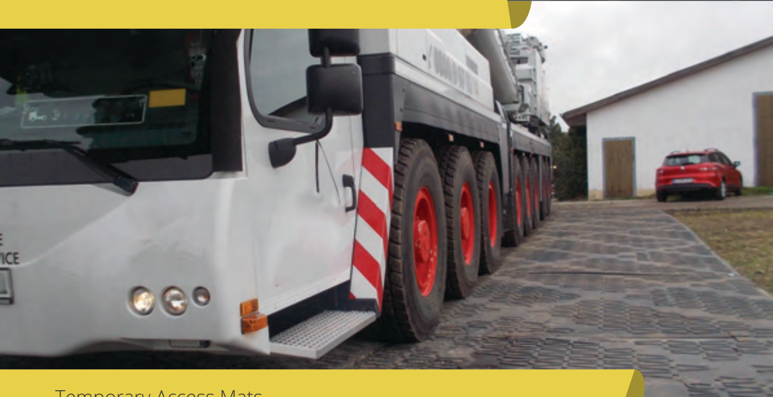
Temporary Access Mats
